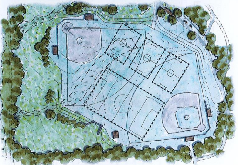
Multi Use Athletic Fields Layout B Softball & Baseball with (1) U10 & (3) U6-8 Fields
