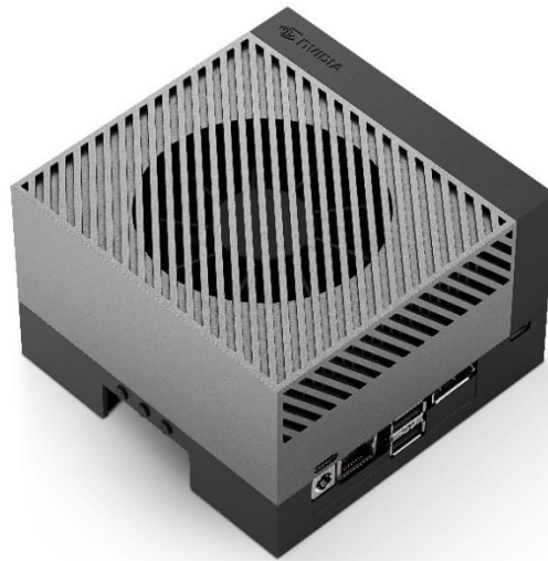
Figure 13: Jetson AGX Orin Developer Kit
