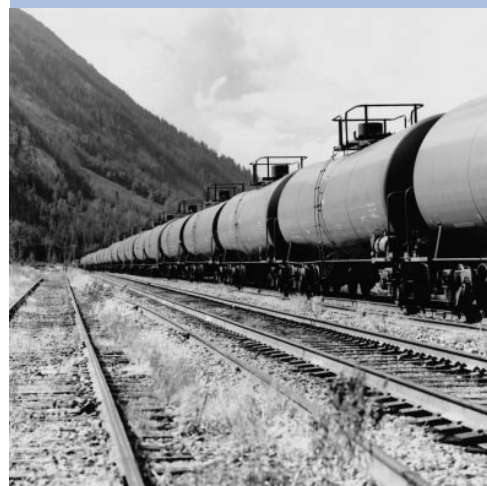
The nation's railroad tank cars are stronger and safer because of Safety Board investigations and recommendations that resulted in tank car headshields, and thermal and puncture protection.
