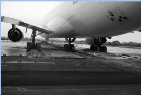
This cargo jet was stopped from running off the runway at New York's LaGuardia airport in 2003. It was stopped by an "arrestor bed"—a cellular concrete structure at the end of the runway that slows the aircraft.
