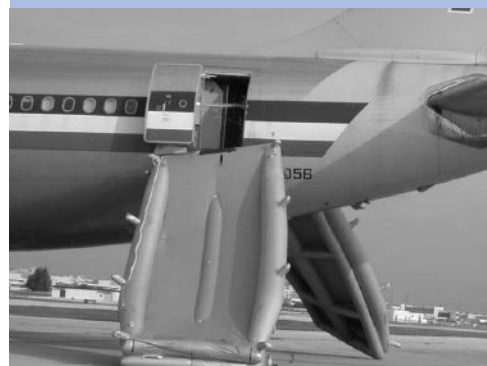
Aircraft evacuation slides have been upgraded to better resist heat from post-crash fires.
