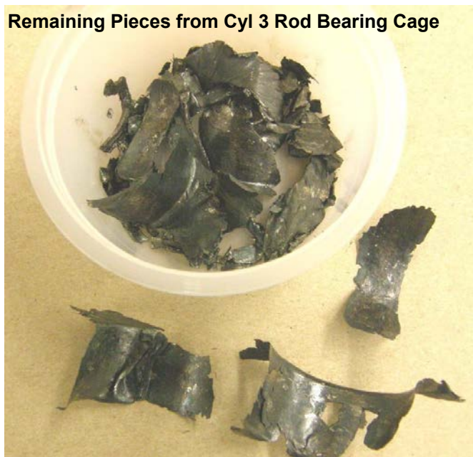
Figure 44: 200HP EFI Bearing Failure Pictures
