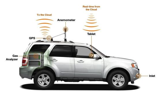
Diagram of vehicle-based advanced leak detection used for distribution systems. Source: Picarro
