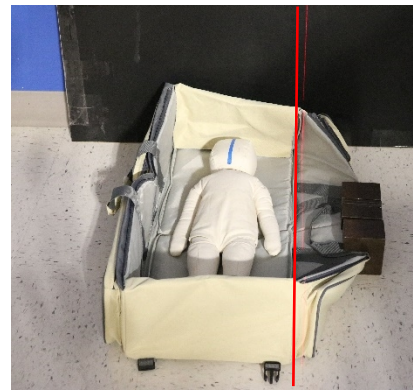
Figure 8b. Cardboard compact bassinet with 23 lb. downward load and 5 lb. horizontal force
