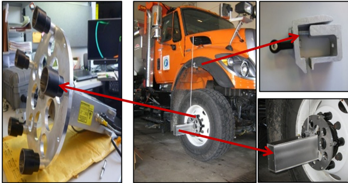
FIGURE 2 Automated test roller designed for vertical displacement measurement: (a) mounting disk; (b) displacement laser device; and (c) details
