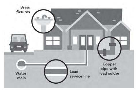
Common sources of lead in drinking water include lead service lines or brass fixtures and plumbing materials with lead solder. When present, a lead service line is the largest contributor of lead in drinking water. Image Source: Elevate Energy.
