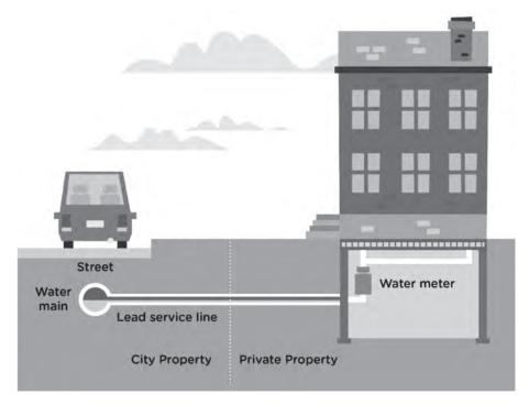
A water service line delivers water from the main in the street to a home or building. These lines may be made of lead if the home or building was constructed prior to 1987. It is important to replace the full lead service line—from the water main to the home—because partial lead service line replacement can increase levels of lead in drinking water. Image Source: Elevate Energy.
