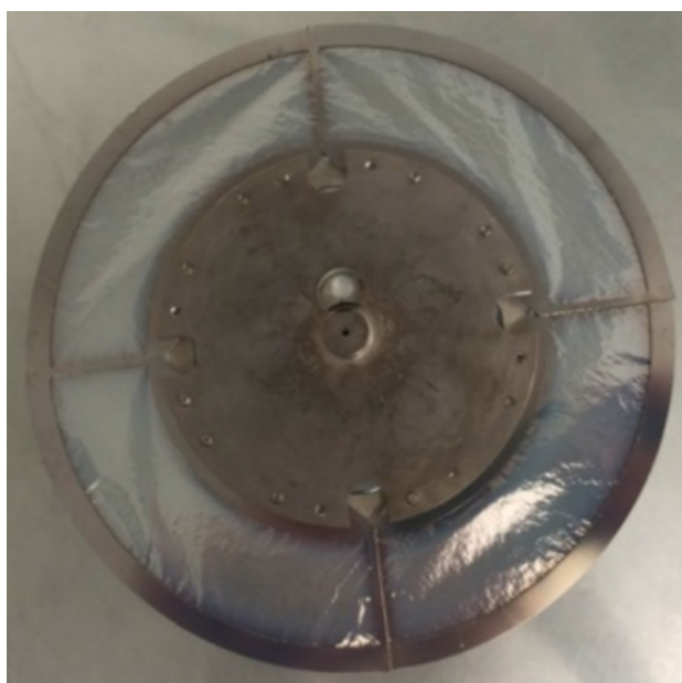
Figure 6.1: ^{209}\text{Bi} target produced via vapor deposition
