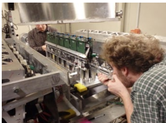
Figure 3: (Left) The target carriage and silicon strip detector arrays used in the kinematically complete measurements of two- and three-body photodisintegration. (Right) Two-dimensional histogram of the energies for the two charged particles detected in coincidence from the photodisintegration of {}^3\text{He} in the HIGS experiment, reproduced from [15].
