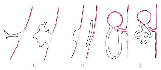
Figure 1: Pairs of scenarios illustrating differences in measured displacement depending on the metric used. Original polylines shown in black, simplified polylines shown in red. (a) approximately equal linear displacement but very different areal displacement, (b) approximately equal Hausdorff distance but very different Fréchet distance, (c) approximately equal shift in areas covered by adjacent polygon features but very different positional displacement of line features.
