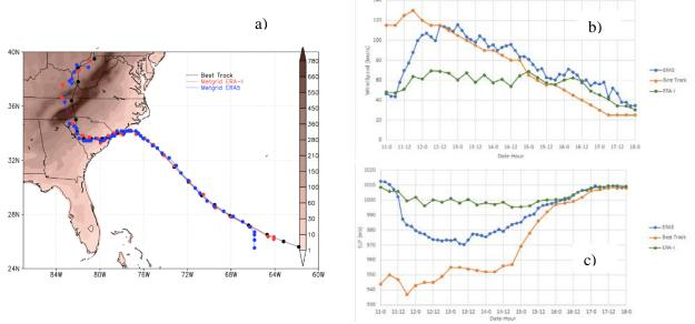
Fig. 2 Comparison of the ERA data with the best track data for: a) track; b) maximum wind; c) minimum SLP.
