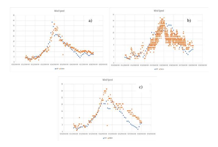
Fig. 4 The wind speed from WRF Week 6 Case 7, in comparison with the stations data, a) Cape Lookout;
